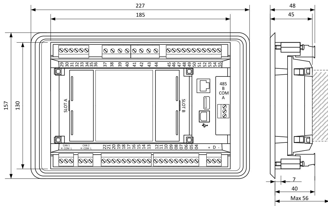
**Note:** The final depth of the controller depends on the selected extension module - it can vary between 41 and 56 mm. Mind also a size of connector and cables (e.g. in case of RS232 connector add about another 60 mm for standard RS232 connector and cable).
