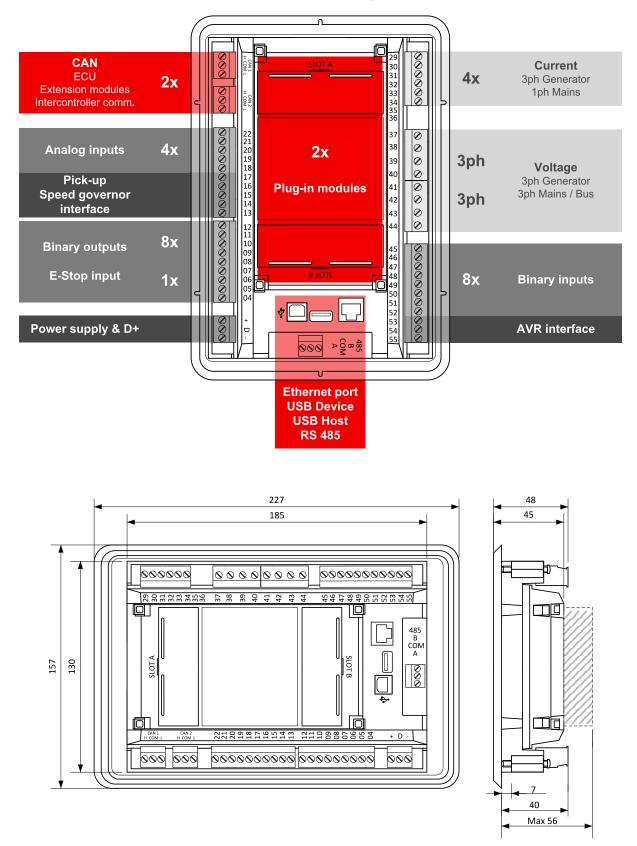
**Note:** The final depth of the controller depends on the selected extension module - it can vary between 41 and 56 mm. Mind also a size of connector and cables (e.g. in case of RS232 connector add about another 60 mm for standard RS232 connector and cable).
